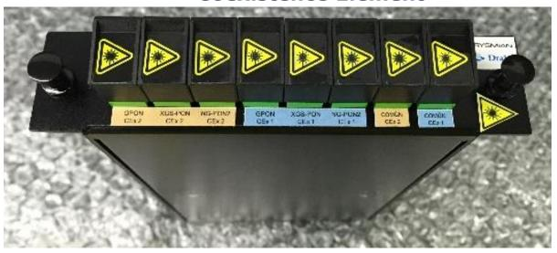
A WDM module or coexistence element is designed to enable the implementation of gigabit passive optical network (GPON) evolutions to XGS-PON and NG-PON2.
