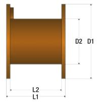
On the above table you can find our most common types of drum. For each one also we provide internal and external dimensions, weight, bulk space and volume. Please consider that a staved drum increase its dimension D1 of 50 mm in total.
