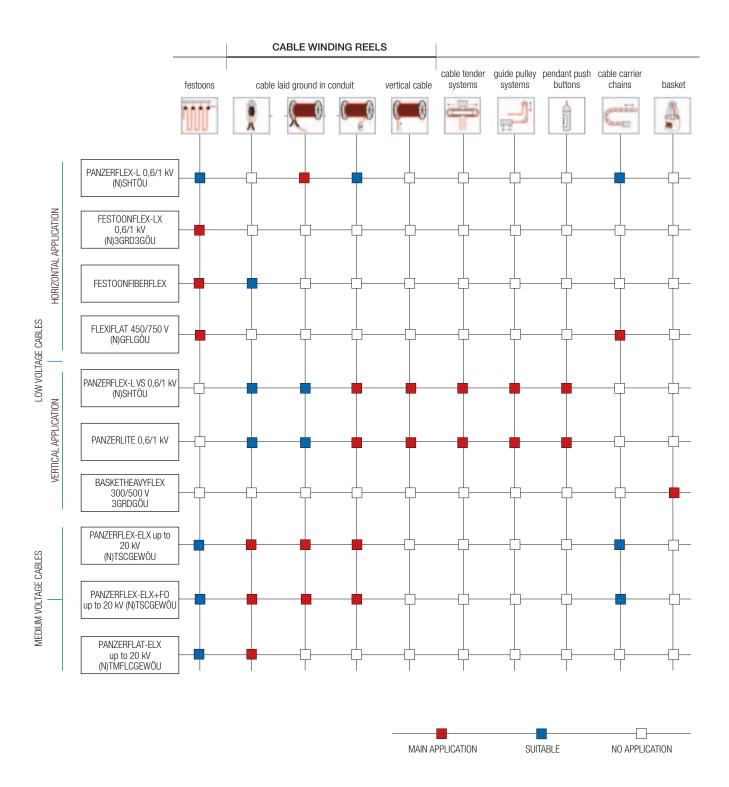
The above table is designed in order to give an easy reference in cable selection for the main mobile equipment application. Please keep in mind that when using this guide all the concurrent factors are to be considered: bending radii, speed, ambient temperature and tension. Even if only one of these parameters stands outside the given data of this catalogue, please contact our sales department for gaining further information.
