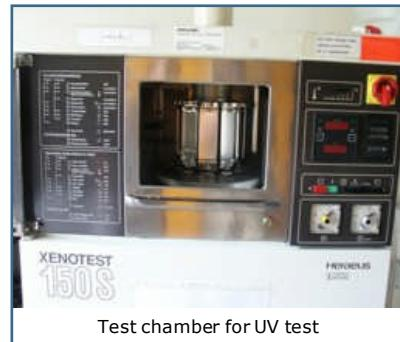
Test chamber for UV test
