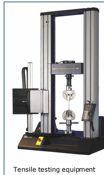
Tensile testing equipment
