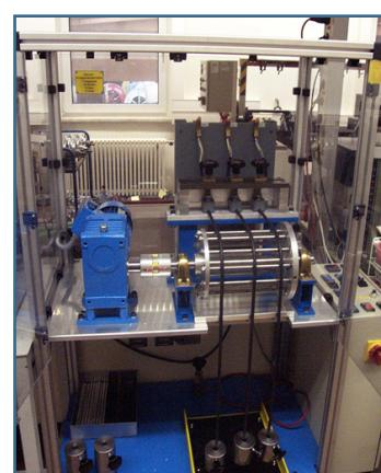
Test cage: sheath against metal/plastic
