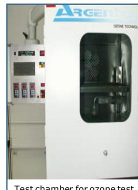
Test chamber for ozone test
